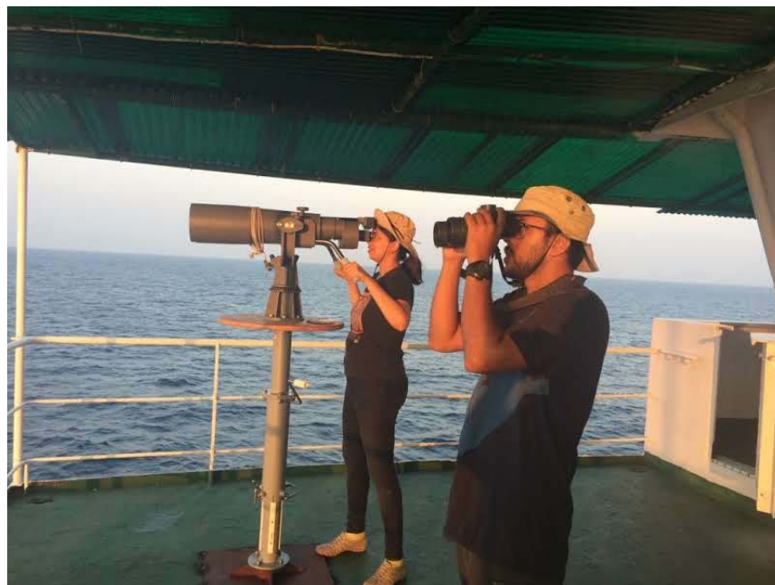
Figure 1. Observers using "Big Eye" binoculars (L) and handheld binoculars (R) to survey for cetaceans at sea.
